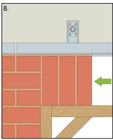
9. Repeat steps 6-8 until all soffit bricks are installed. Install SDB restraint ties as work progresses, typically at 450mm horizontal centres, ensuring that each tie is completely covered with mortar.
