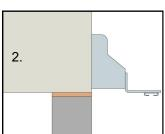
2. Install masonry support system in accordance with our installation guidance and drawings. The Hanger Tie system uses a support angle with a channel, normally 36/8, welded to the underside.
