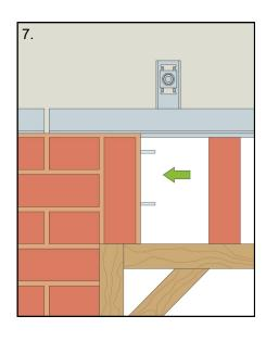
7. Push the next brick onto the dowelled Hanger Tie.
