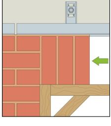
11. Once mortar has achieved design strength, temporary support may be removed and brickwork may be pointed as necessary. (Check with your Structural Engineer if unsure).
