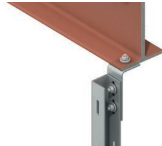
Top Connection of a WP3 Windpost to the Underside of a Steel Beam
