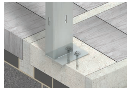
Base Connection of a WP2 Windpost to a Concrete Infill in the Top of a Beam and Block Floor
