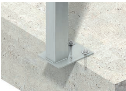
Base Connection of a WP3 Windpost to the Top of a Concrete Slab
