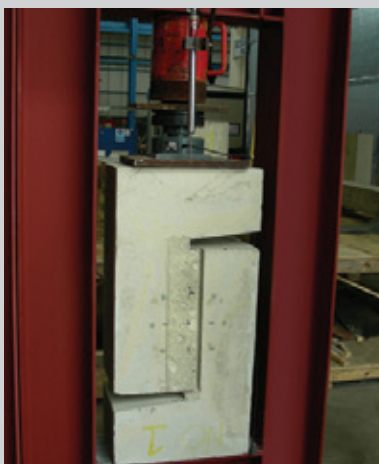
Longitudinal shear test arrangement with Ancon Eazistrip cast into one side of the joint. The load was applied by jack through the test frame.
