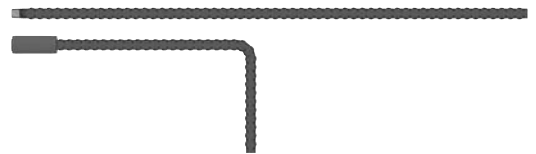
Figure 3: Starter bar system. Top - male component; bottom - female component.
