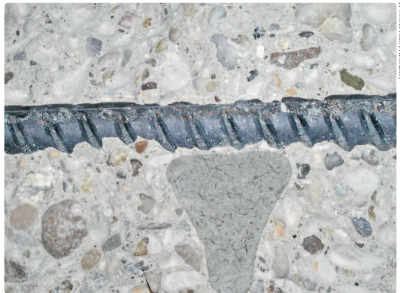
Figure 1 above: Extruded fibre concrete spacers have a tested and proven watertight bond to concrete.
