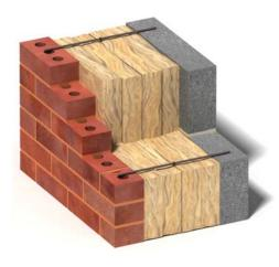
crossing the cavity they act as a thermal bridge. Generally speaking, the wider the insulated cavity, the more substantial the Wall Tie needs to be and the greater the effect the tie will then have on the thermal efficiency of the wall.
