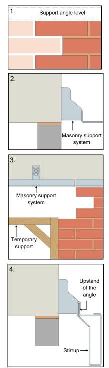
1. Build brickwork up to support angle level on each side of the opening, ensuring that the top three jamb bricks on one side of the opening are left out to allow the installation of the last soffit brick.
