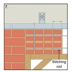
7. 300mm long stitching rods should then be fed through the brick cores as shown, allowing for an overlap of approximately 75mm into the cores of the fourth brick.
