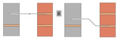
A plastic sieve may be used to retain resin and is particularly useful in perforated brick or hollow blockwork. A 12mm hole is required to fit the sieve.
