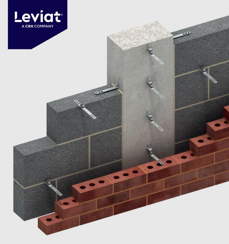
Acoustic wall ties and frame cramps for connecting the leaves of a cavity wall while minimising the transfer of airborne noise and vibration
