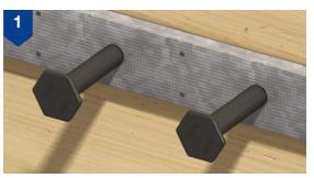
Nail the KSN Anchor Box to the formwork. The wall reinforcement is installed to which the anchors are tied. The concrete is cast and once it reaches sufficient strength, the formwork is removed to reveal the steel cover.
