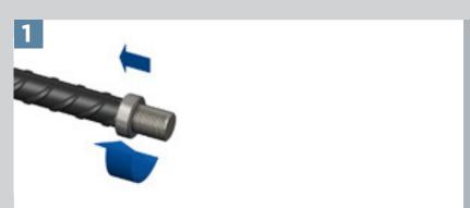
Run the locknut onto the fixed bar.
