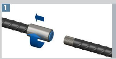
Run the coupler to the end of the thread on the fixed bar.
