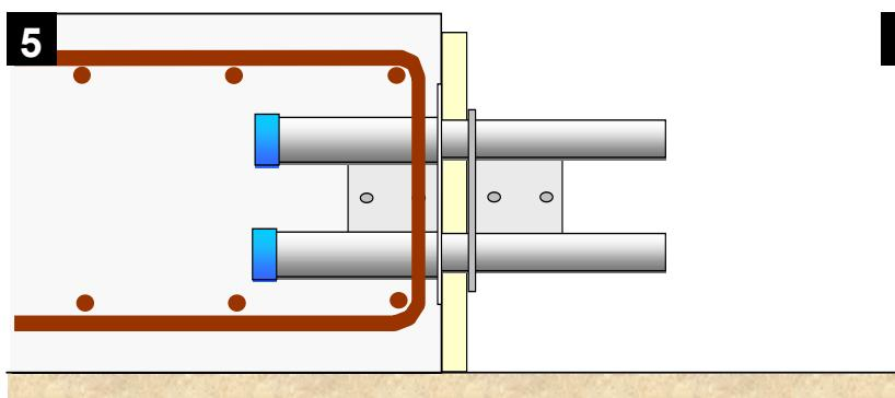
**5** Push the dowel component through the filler until it is fully located in the sleeve
