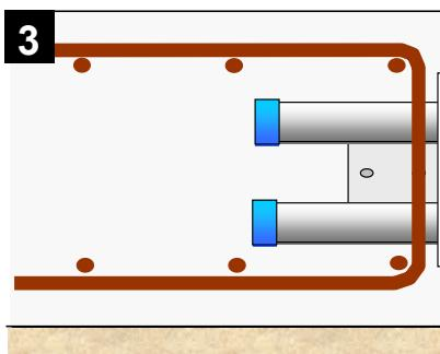
**3** When the concrete has achieved sufficient strength, strike shuttering and peel off or puncture the label
