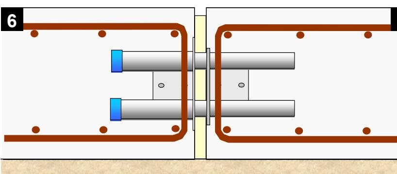
**6** Fix the local reinforcement around the sleeve and pour the concrete
