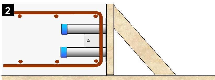
**2** Fix the local reinforcement around the sleeve and pour the concrete
