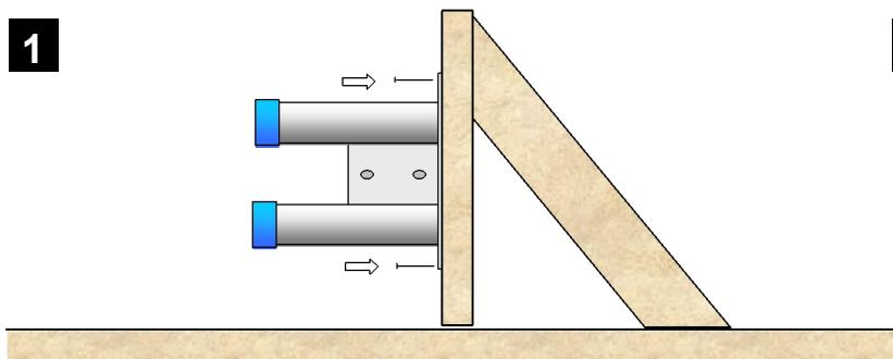
**1** Nail sleeve to formwork. Do not remove sticky label, this prevents ingress of concrete into the sleeve
