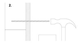
Hammer the tie, through the insulation, and into the blockwork to the correct embedment.
