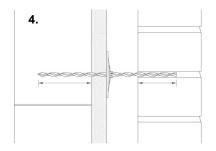
Build into the bed joint of the outer leaf ensuring the tie is surrounded by mortar.
