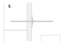
Install a black Teplo Clip to restrain the insulation.
