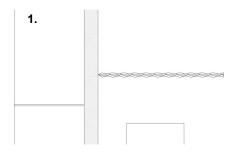
Keep the brickwork one course clear during installation of the ties. Position the tie against the inner leaf so that the outer end will be located in the bed joint of the external leaf.
