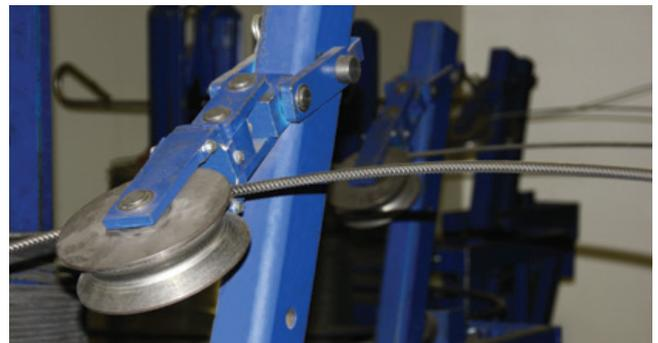
Decoiler Diverter Pulley
