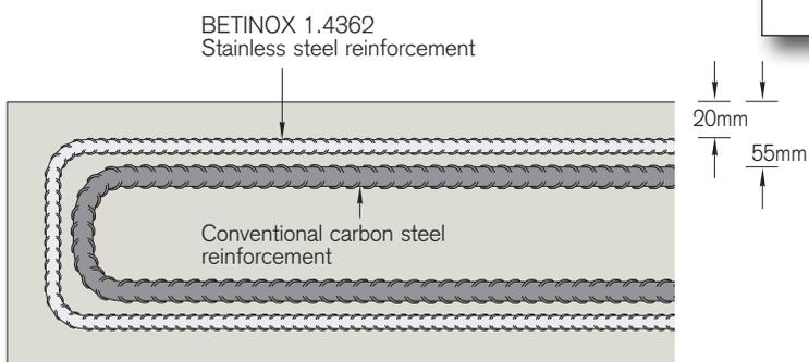
Comparison of concrete cover required for traditional carbon steel and BETINOX stainless steel reinforcement
