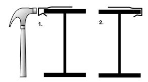
Plan View Application - The Hammer-On Section MUST be fixed to alternate sides of the flange (225mm Vertical Centres) as work progresses
