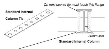
The tie must be in contact with one flange; the choice of flange should alternate at each course
