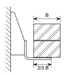
To cater for minor deviations in the position of the structural face, the position of the masonry wall on the support angle can be adjusted. Ideally, the design bearing width of the masonry wall on the angle is at least two thirds of the width of the wall. In practice, this can be reduced, but the advice of the support system manufacturer should be sought.
