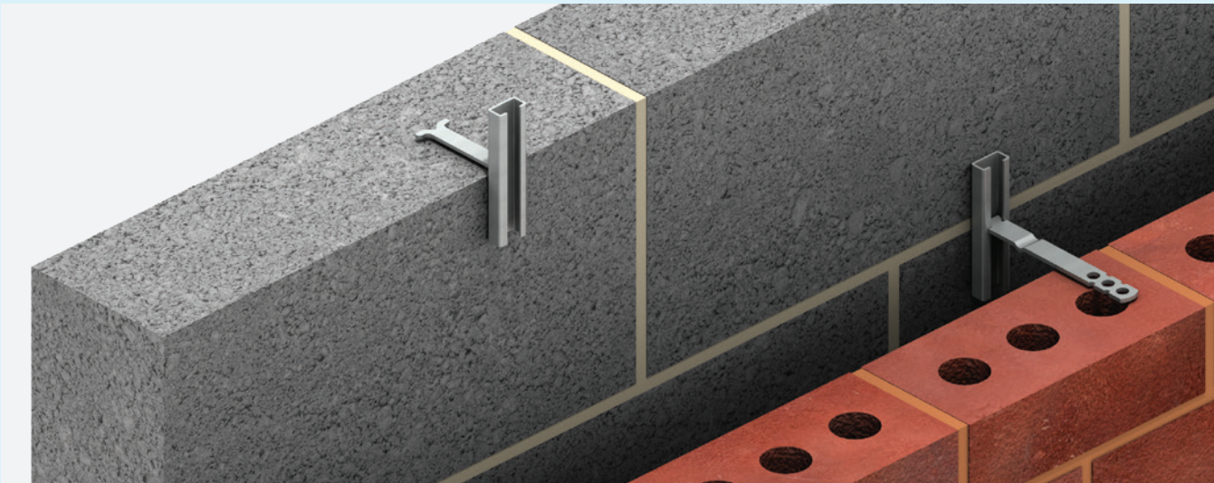
Ancon Fastrack Channels 100mm long with Ancon SD28 Tie
