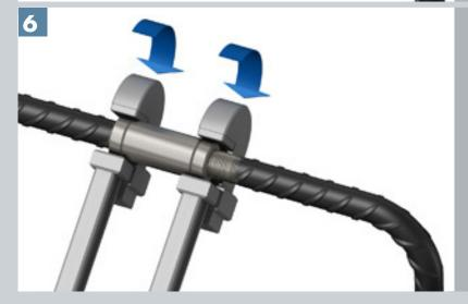
Tighten the locknuts against each other using a pair of wrenches.
