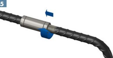
Rotate the locknut along the continuation bar to abut the coupler.
