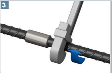
Tighten the joint using a wrench on the continuation bar.
