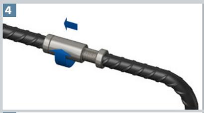
Run the coupler from the continuation bar onto the fixed bar.
