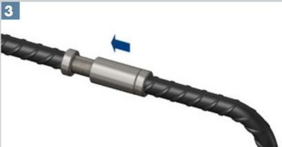
Position the continuation bar with the coupler against the end of the fixed bar.
