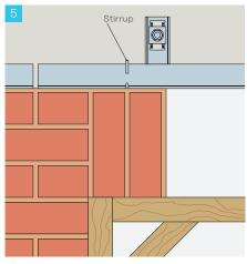
Offer a brick either side of the stirrup, filling the joints completely with type M12 (or equivalent) fresh mortar. Ensure the void between the underside of the support angle and the top of the hung brick is tightly packed with mortar.
