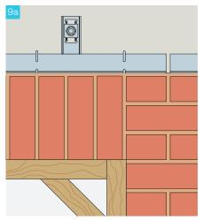
Install final jamb bricks, filling each joint with fresh mortar.
