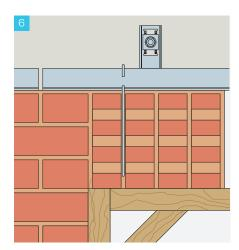
Fill the cores of the bricks completely and lay another two bricks adjacent to these, filling each joint with type M12 (or equivalent) fresh mortar.
