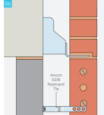
Clip the next stirrup onto the support angle, and repeat steps 5-7 until all bricks are installed (8a). Install Ancon SPB Restraint Ties as work progresses, typically 450mm horizontal centres, ensuring that the tie is completely covered with mortar (8b).
