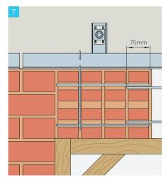
300mm long stitching rods should then be fed through the brick cores as shown, allowing for an overlap of approximately 75mm into the cores of the fourth brick.
