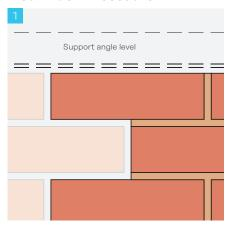
Build brickwork up to support angle level on each side of the opening, ensuring that the top three jamb bricks on one side of the opening are left out to allow the installation of the last soffit brick.
