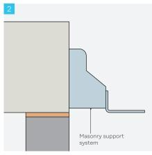
Install masonry support system in accordance with our installation guidance and drawings.
