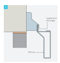
Clip the first stirrup onto the support angle. This should be vertical and hung from the upstand of the angle.
