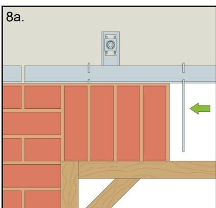
9. Install final jamb bricks, filling each joint with fresh mortar.
