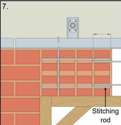
7. 300mm long stitching rods should then be fed through the brick cores as shown, allowing for an overlap of approximately 75mm into the cores of the fourth brick.
