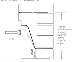
Before any further courses are built, the mortar should be allowed sufficient time to cure for the ties to take the restraining load as the brickwork proceeds. The time period will vary, but should be at least two days, and will be more if the mortar has additives to extend its workability and/or in particularly cold weather.
