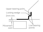
on the compressible filler. If the fixing face is uneven, low points may need to be packed to ensure the backs of the brackets are in-line. Any packs should be fixed securely.
