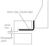
will need to be set higher to limit the mortar bed to a maximum of  $5\,\mathrm{mm}$ .
