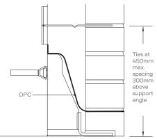
Before any further courses are built, the mortar should be allowed sufficient time to cure for the ties to take the restraining load as the brickwork proceeds. The time period will vary, but should be at least two days, and will be more if the mortar has additives to extend its workability and/or in particularly cold weather.
