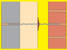
250mm long for cavities from 101-125mm 275mm long for cavities from 126-150mm
