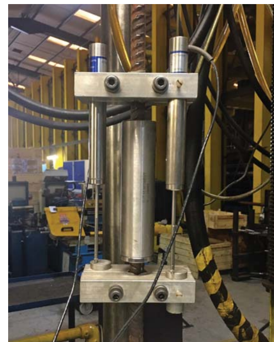
Ancon HM half-grout sleeve under test.
