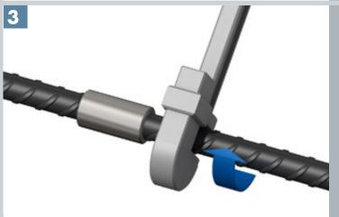
Tighten the joint using a wrench on the continuation bar. After tightening there should be no more than 2-4mm of exposed thread, depending on the diameter of the rebar.
