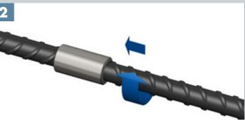
Remove the thread protector from the end of the coupler. Position and rotate the continuation bar such that the thread fully engages within the coupler.
