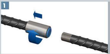
The CXL Type A coupler is rotated to the rear of the thread on the fixed bar, then locked tight. The bar end should be central within the coupler.
