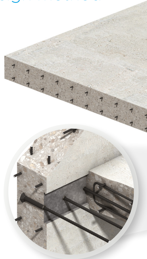
KSN Anchor Box, a single row of KSN Anchors positioned along the slab section centreline. Bartec Plus threaded reinforcing bars, also from Ancon, complete the connection
