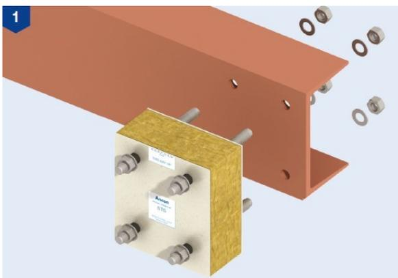
The SSTS/STS Balcony Connector should be orientated so that the label indicating the uppermost face is correctly positioned and is facing out of the building.
