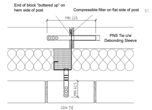
Fig. 2 Ties for the inner leaf (Movement joint)
