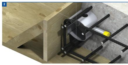
After laying the required reinforcement and a final check to ensure that there is sufficient reinforcement and concrete cover, the concrete can be placed in the formwork. This completes the installation of the sleeve component.
