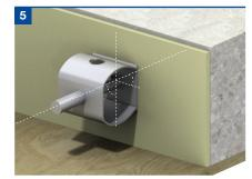
Now press the dowel component through the joint filling material into the installed sleeve as far as it will go. To prevent the dowel component from shifting during concreting, the sleeve is equipped with a small pinch that fixes the dowel component in the installed state. To prevent crushing when inserting the dowel component, light tapping may be necessary.
