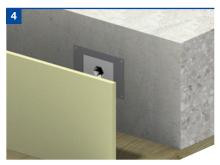
Now the joint can be lined with joint filling material of suitable thickness.
