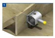
The sleeve component is fixed to the formwork with nails, aligned according to the load direction. Check that the minimum edge and centre distances have been observed. The sticker protects the sleeve component from the penetration of concrete or cement milk and should not be damaged at this stage.
