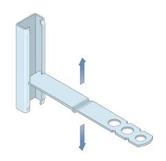
Press the safety end of the tie firmly down into a layer of fresh mortar and cover with another layer of fresh mortar prior to laying the next brick on top. The starting position of the tie should be 15mm from the base of the channel. Installed ties should be clear of mortar droppings.
