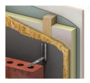
The Ancon TFMT7 is designed to tie masonry (typically brickwork) back to a structural timber frame whilst accommodating differential movement. The system comprises a 90mm long channel, SD25 strip tie and Ø6x50mm hex head coach screw. The TFMT7 can be manufactured to suit any cavity from 50mm to 150mm.
