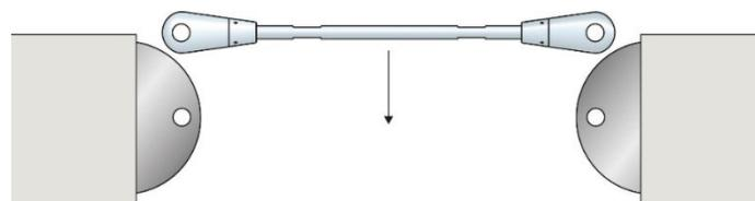
In systems that have a disc, the bars should be installed in a sequence so that the fork towards the disc is installed last.
