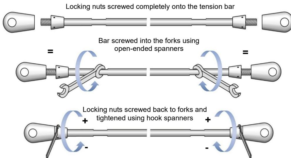
No thread should be visible past the locknut. To make adjustments to the length of the system, to achieve a specific pin-to-pin dimension, unscrew couplers (if used) and then unscrew fork ends. Ensure adjustment is distributed along all adjustable components to make certain no thread is showing across the entire assembly.
