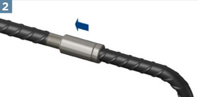
Position the continuation bar with the coupler against the end of the first bar.
