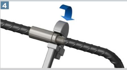
Hold the rebar in the required orientation and with a wrench tighten the locknut against the coupler.
