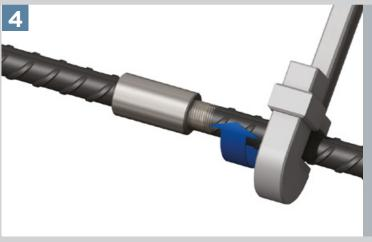
Using a wrench, rotate the continuation bar to lock the two bar ends against each other within the coupler.
