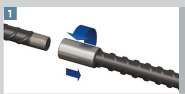
Screw the CXL Type B system coupler to the rear of the thread on the continuation bar.
