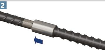
Position the continuation bar with the coupler against the end of the first bar.
