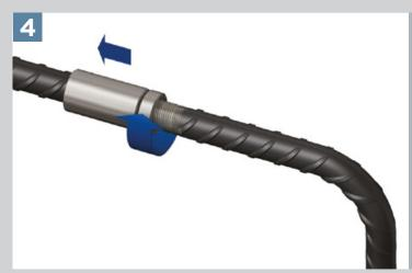
Rotate the locknut along the continuation bar to abut the coupler.
