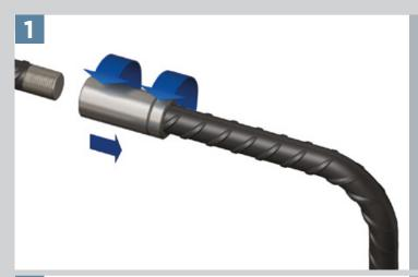
Screw the locknut followed by the CXL Type C system coupler to the rear of the thread on the continuation bar.
