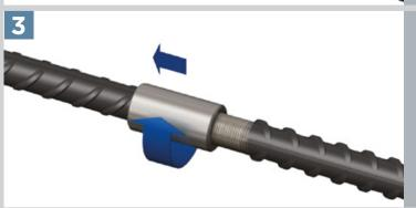
Rotate the coupler from the continuation bar to engage against the rear of the thread on the opposing bar and lock tight.
