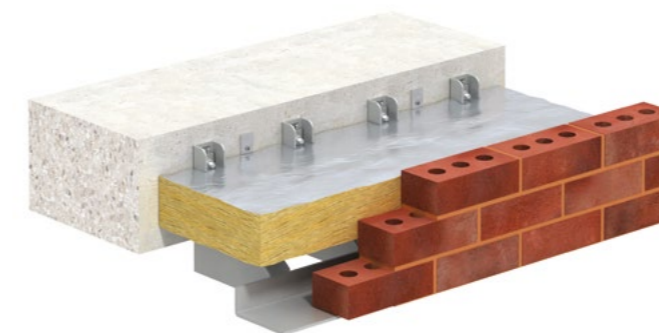
Cavity barrier fully penetrated by Ancon MDC Masonry Support System
