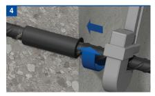
To ensure correct installation, tighten the joint to the specified torque using a calibrated torque wrench on the continuation bar. Tightening torques are shown in the table below.
