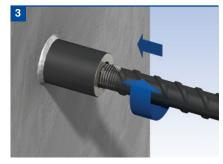
Rotate the bar into the coupler until tight.
