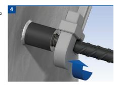
To ensure correct installation, tighten the joint to the specified torque using a calibrated torque wrench on the continuation bar. Tightening torques are shown in the table below.
