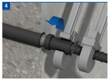
Using a torque wrench tighten the male component on the continuation bar to the specified torque, whilst holding the continuation bar with a second wrench.
