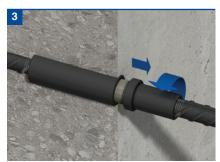
Run the male component and locknut onto the continuation bar until fully engaged.
