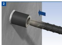
When ready to extend, remove the plastic end cap and position the continuation bar into the sleeve.
