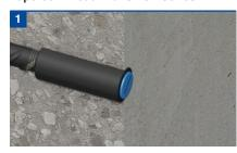
The coupler is normally supplied fixed to a reinforcing bar, ready to be installed and cast in concrete
