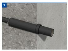
The female section of the positional coupler is normally cast flush in the concrete. The installer must take care to protect the internal threads and prevent the ingress of concrete. Once cast and ready to extend, the male end complete with locknut can be screwed into place.
