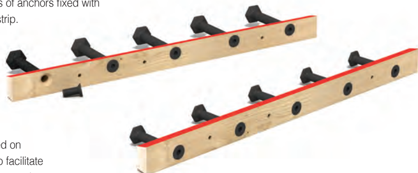
Tapered timber strips simplify installation, create a shear key and increase anchor embedment
