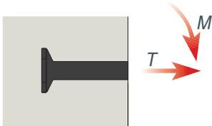
From the tests conducted to determine the direct pull out capacities of KSN Anchors (see page 6), we identified a potential increase in anchor performance when the compression part of the moment couple lies within the pull out cone.
