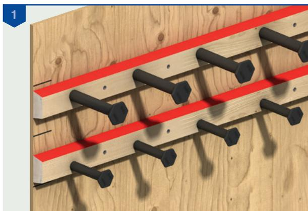
The timber carrier supporting the anchors is positioned against the formwork at the required location of the adjoining slab, orientated to the instructions on the label which indicates that the coloured side should face up. The timber is fixed to the formwork with nails. It is important that the strip is set to the correct position within tolerance, is the right way up and fixed to prevent any movement during concreting.
