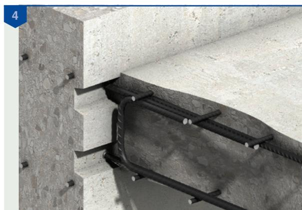
Slab reinforcement should be installed to the Engineers details. The slab is cast to complete the application.
