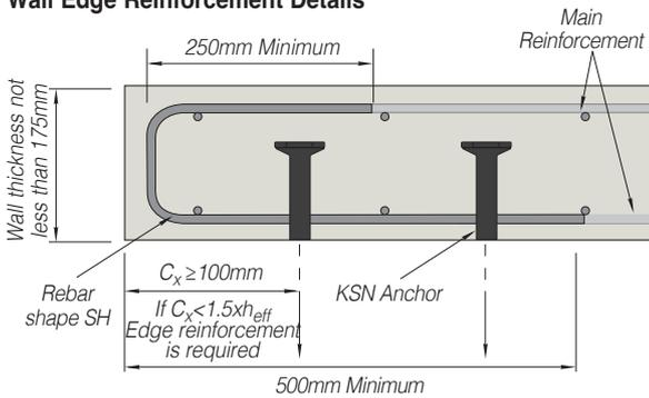
**Reinforcement:** Minimum edge reinforcement, 12mm diameter Grade B500B
