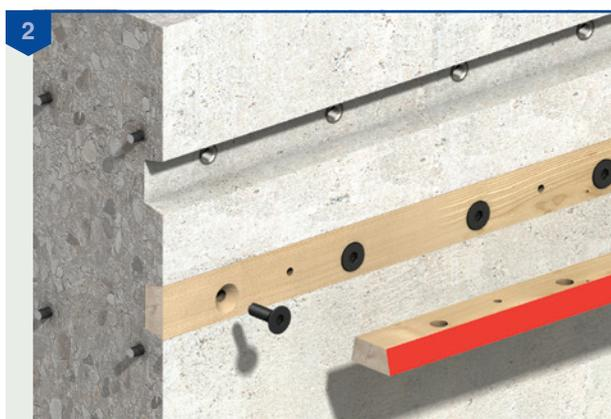
Other wall reinforcement should be installed to the Engineer's details, based on our recommendations. The concrete is then cast and once it has reached sufficient strength, the formwork is removed to reveal the face of the timber strip with the protective tape.
