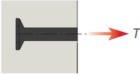
The direct pull out strength of anchors embedded in concrete has been the subject of extensive research over many years. To determine the direct pull strength of KSN Anchors, we commissioned a test programme at Heriot Watt University, UK. The test results and subsequent analysis aligned closely with established formula for the pull out strength of anchors. The direct pull out strength is based on a model with a break out prism angle of approximately 35 degrees. See Fig A.
