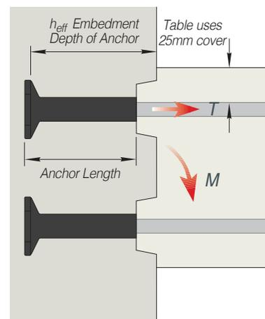
**Notes:** Refer to key design considerations on page 8. In addition, the tables assume no close edges and a cover to the top and bottom reinforcement connecting to the anchor of 25mm. For other cover, please contact Leviat. **Bold** figures indicate performance equal to or greater than reinforcement design resistance. If not bold, anchor resistance is limited by the concrete design resistance and we recommend the use of secondary wall reinforcement (see page 17).
