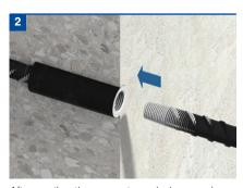
After casting the concrete and when ready to extend, remove the plastic end cap (and nailing plate where appropriate) from the coupler. Position the continuation bar in the sleeve and rotate the bar into the coupler.
