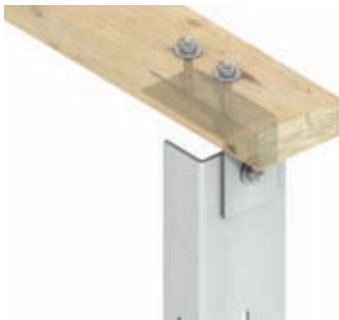
Top Connection of a WP2 Windpost to the Underside of a Timber Wall Plate
